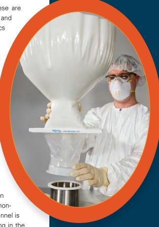
It is easy for traditional style single use bags to become contaminated on the outside as product is spilled or overflows, or simply settles from the surrounding air. DoverPac's® EZ BioPac™ has a protective outer skirt that covers the outside of the bag during filling, reducing surface contamination and making sealing and handling a cleaner process.
